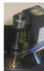
Target switch and cam for close valve
