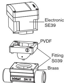
The flow controller 8039 is built up with an electronic module SE39 associated to a fitting S039 with integrated measurement paddle-wheel.
